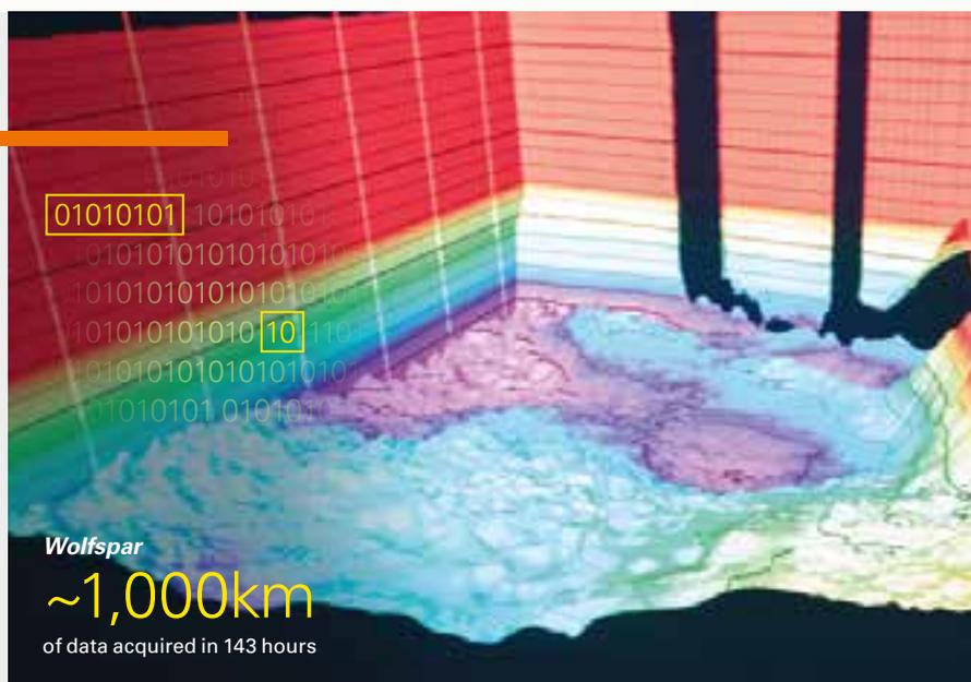
and Schlumberger. The project aims to move beyond the existing limitations of bulky, heavy and expensive onshore seismic equipment, and at the same time provide better images of the reservoir. Following successful initial field trials in Norway and Abu Dhabi in 2017, the 'nimble node' system was used to safely acquire 3D seismic data in the challenging climate of West Siberia in 2018. Early images show better data quality compared to conventional equipment, with fewer people
